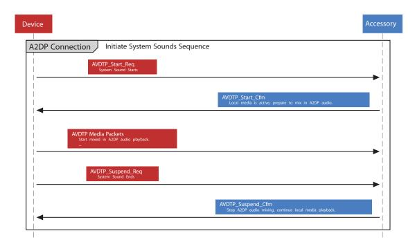
Figure 2-2 Initiate System Sound (e.g. turn-by-turn directions)
